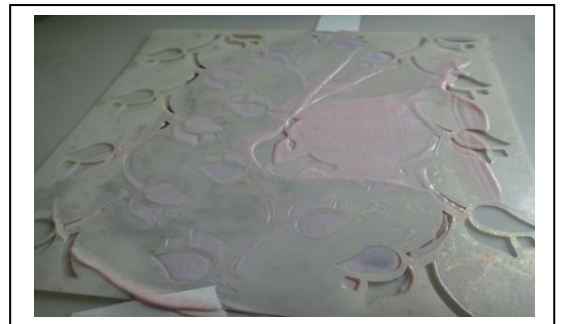
Now place the paste onto the mask & drag the paste over the mask. Remove any excess paste once it's all smooth over the mask.
